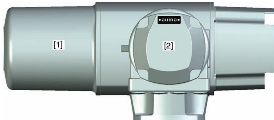
Figure 79: Access to fuses
