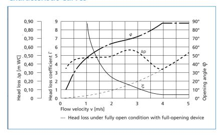
Measured curve of an **ERHARD** Tilting-disc Check Valve DN 500, PN 10, with weight-loaded lever for installation into a horizontal water pipeline.
