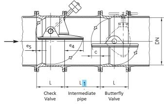
**Attention!** Installation must be effected in such a way that the weight-loaded lever of the Check Valve is on the left seen in flow direction and that the gearbox of the Butterfly Valve is on the right, seen in flow direction. Thus, there will be no collision between weight-loaded lever and gearbox.
