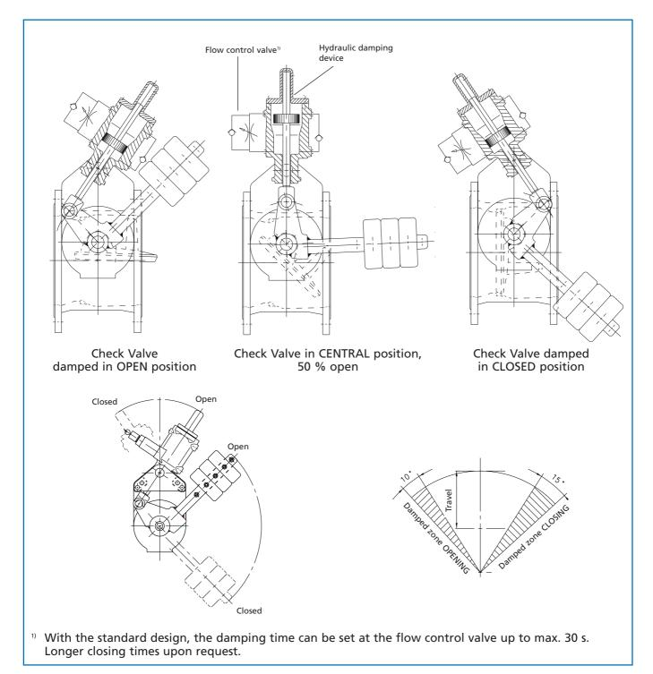
If the standard types are equipped with hydraulic damping cylinder, due to shaft dimensioning and material, the admissible back pressure is limited as follows:
