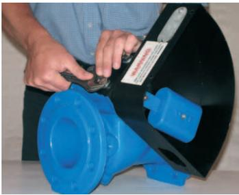
Tighten the bolts connecting the bonnet and body.
