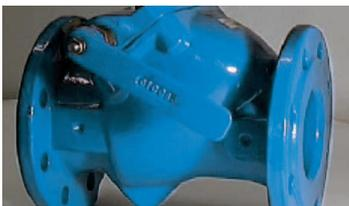
Mount the lever. Tighten nut and washer firmly. Note: The lever can be mounted in 6 positions due to the inside hexagon shape of the lever. The position of the lever should be giving maximum force on the disc, when in closed position.
