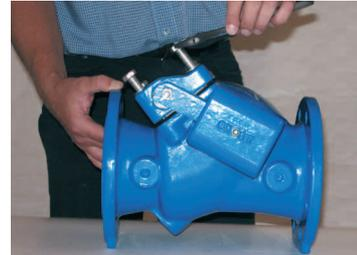
Loosen and remove the two bolts closest to the lever and weight. Washers are to be used again.
