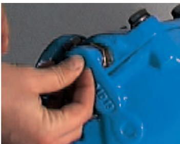
Mount the lever on the closed valve. Choose position of lever in such a way that the spring is relaxed when connected to the bracket. Tighten nut and washer firmly.
