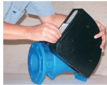
Mount the protection guard to the back plate with the screws
