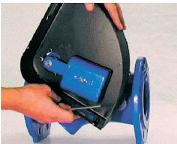
Adjust the back plate according to the position of the lever and weight. The back plate is positioned correctly when there is approx. 15 mm between weight and back plate.
