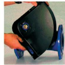
Mount back plate and adjustment plate on the bracket. Do not tighten the screws.
