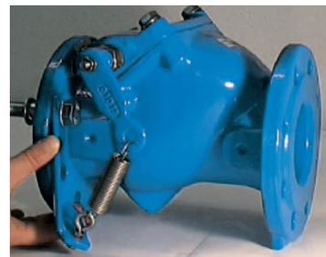
Before mounting the spring lever kit, the valve is to be fully installed in the pipe system. Mount the spring thus connecting the bracket and the lever. When the valve is in closed position the spring should be relaxed.
