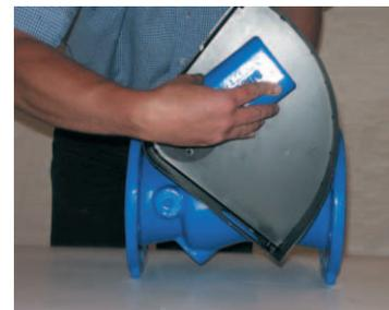
Make sure that there is enough space between the back plate and the lever and weight.
